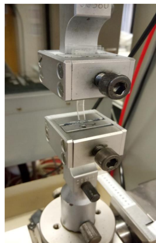
Fig.2 A total of 8 tensile tests were carried out. This gave an average modulus of elasticity of 1.56 MPa for the stiffest gel.
